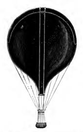
VALVES are fitted at the neck and at the top of a balloon.
